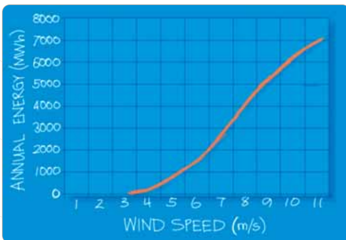
Annual energy output (MWh/year) relative to mean annual wind speed (m/s) for a 1.65MW wind turbine.
