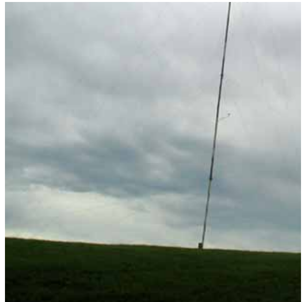
Research masts are installed to measure wind speed and direction.
