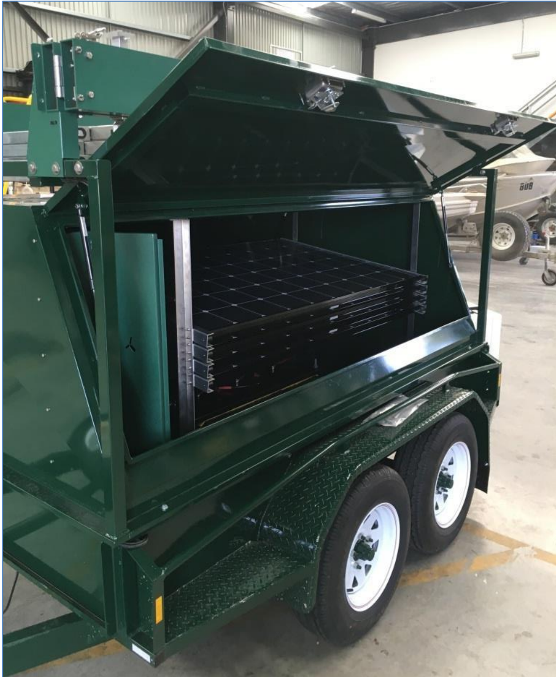
Internal Solar Panel Racking above Battery Bank for Ease of Transportation
