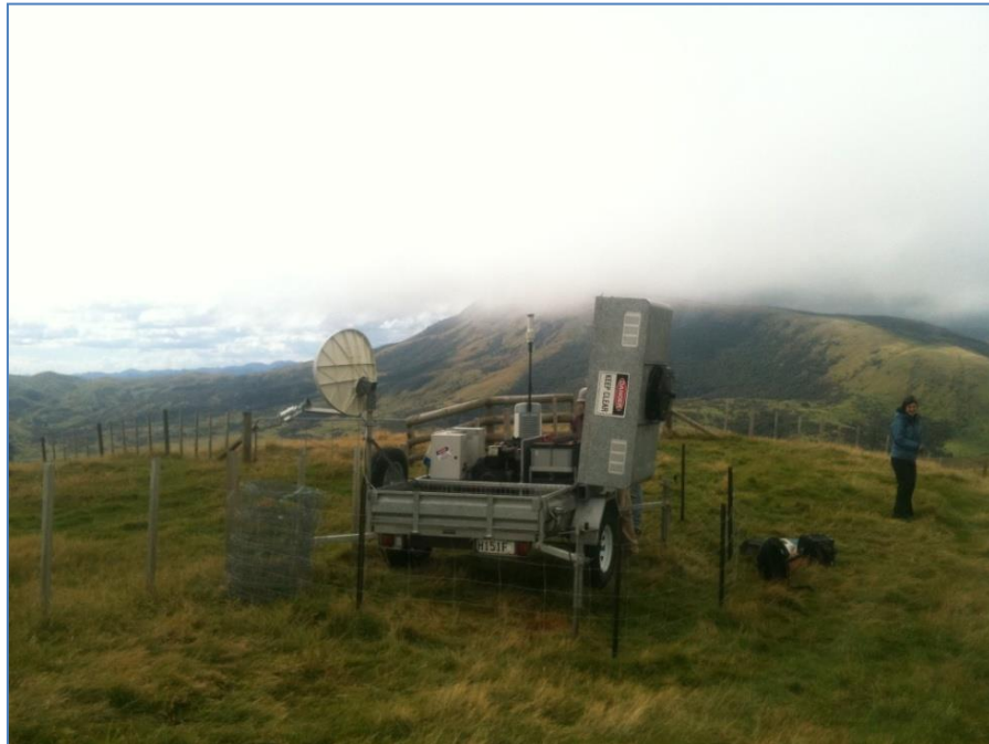
Trailer Mounted Power Pack for ZephIR V1
