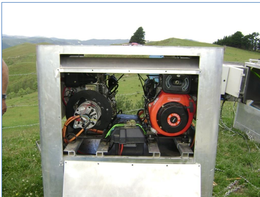
Internals of Optional Generator Enclosure (2 x Diesel engines for Customer Specified 98% Availability and Reliability)
