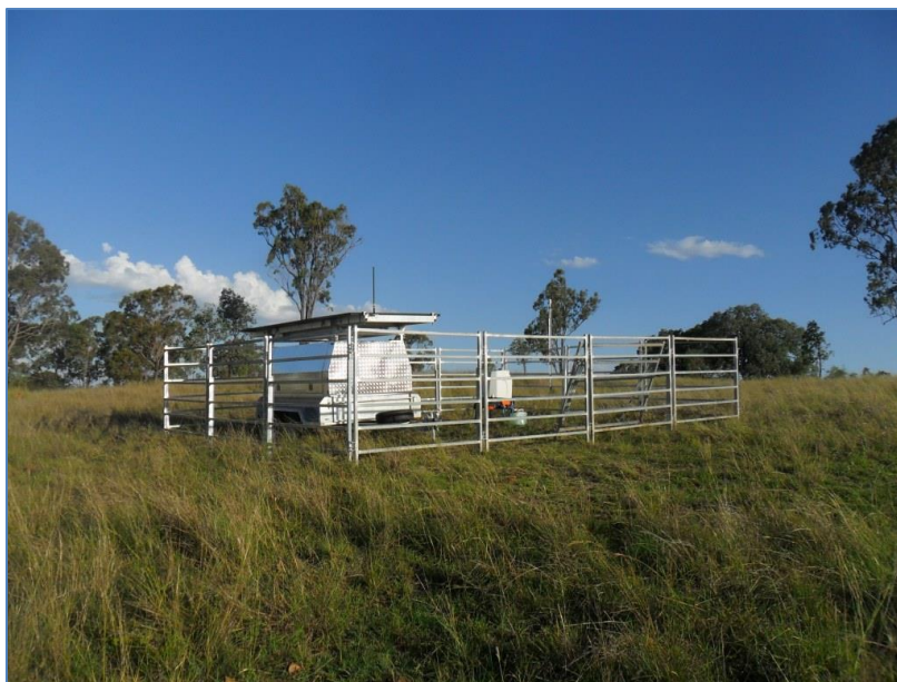
An example of an Energy3 solar-powered remote power supply trailer and LiDAR
